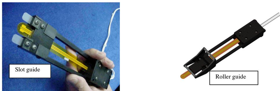
**Figure 2:** Custom wand holders with adjustable insertion length and slot guides (left) or roller guide (right)
