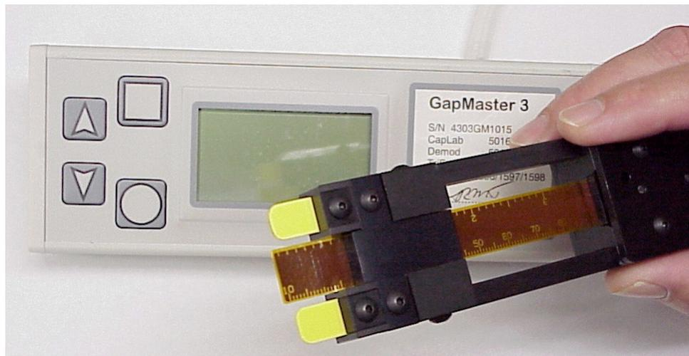
*Figure 3:* Complete Gapmaster 3 Portable Shop Floor System
