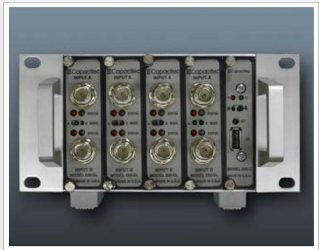
Model 208 (8-channel rack) with (4) 520-XL amplifiers and (1) 200-C oscillator card
