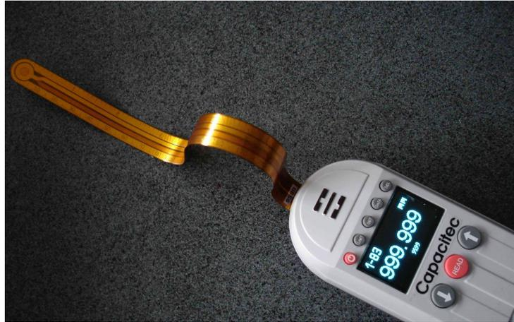
*Figure 3. Gapman Gen3 with flexible wand with dual capacitive non-contact sensors*
