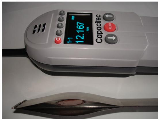
*Figure 5: Spring contact wand for gap measurement of non-conductive targets*
