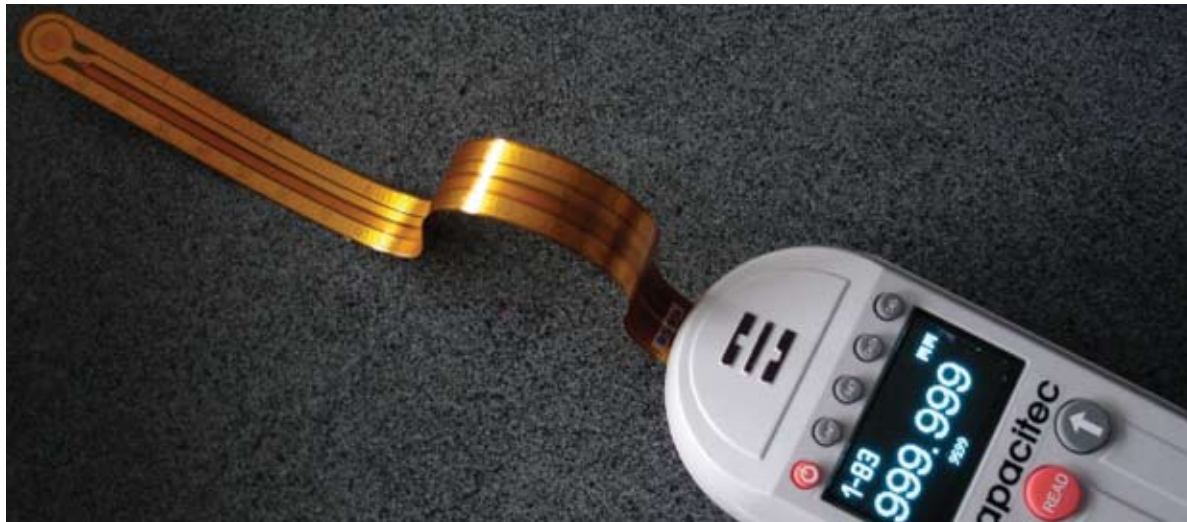
Left: Gapman Gen3 with flexible gap sensor wand
