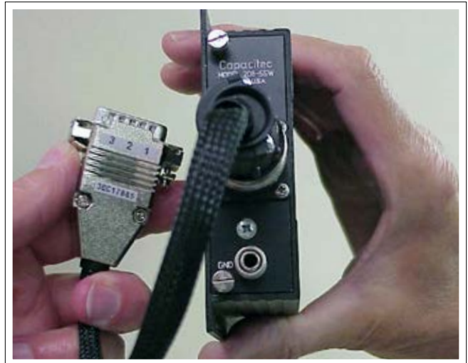
3 sensor input view with TRW/Souriau connectors
