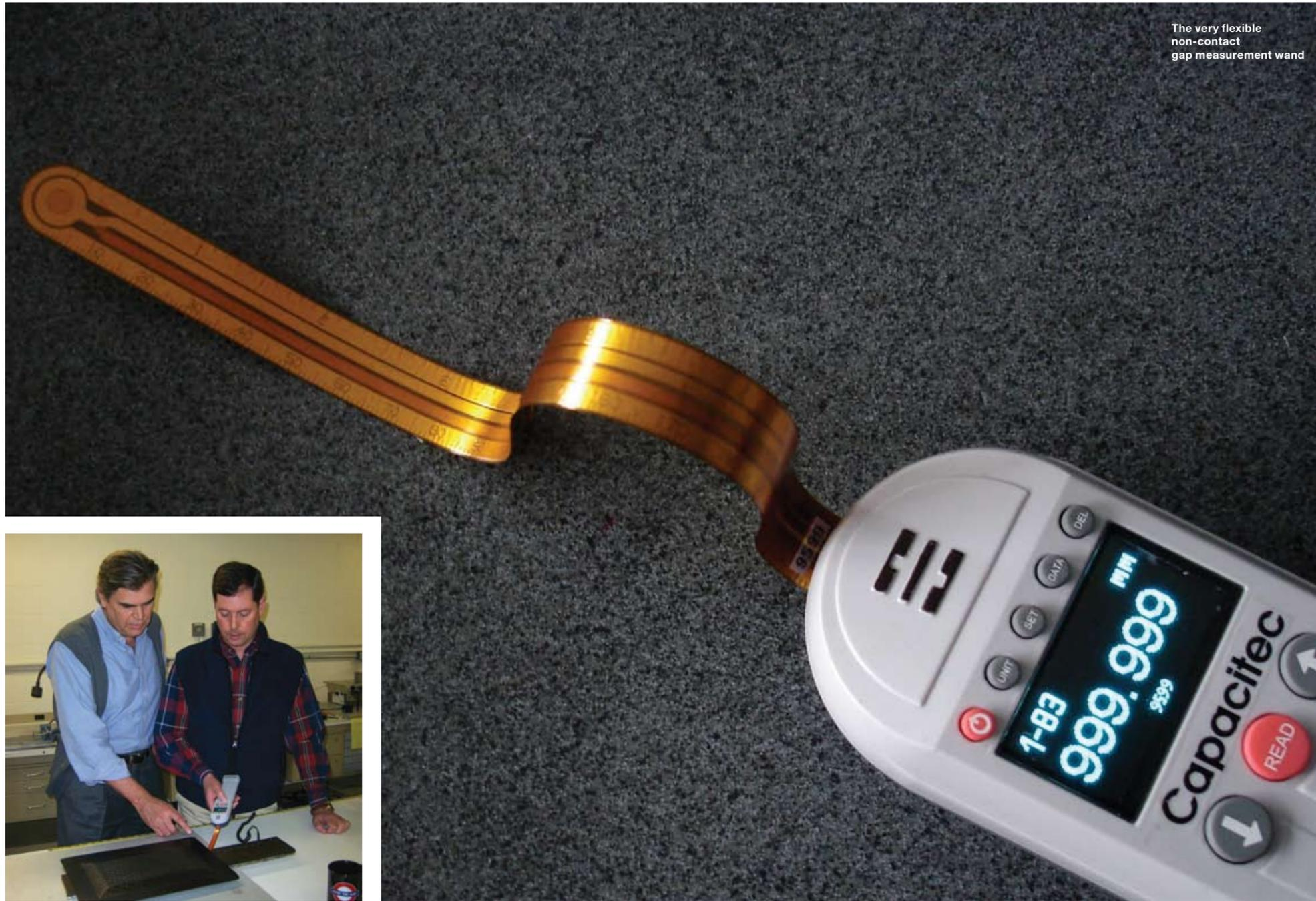
The very flexible non-contact gap measurement wand
