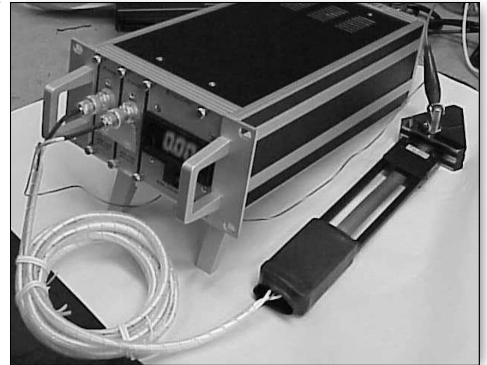
Two channel system with instrumentation, wand holder and calibration block
