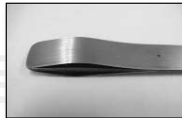
Contact type wand for use in measuring odd shaped gaps
